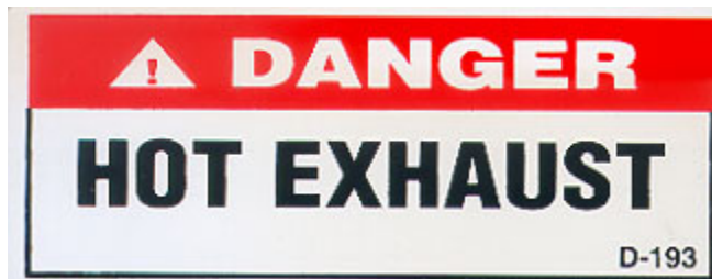
090193 Right Frame Rail ahead of exhaust pipe
