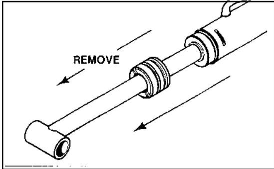
4 Inspect the piston and the bore of the cylinder tube for deep scratches or galling. If damaged, the piston and cylinder tube must be replaced.
