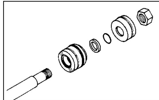
3 Secure the cylinder rod (mounting end) in a vise, with a support at its center. Torque the nut to the amount
