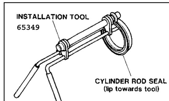
Rotate the handles on the tool around to wrap the seal around the end of the tool.
