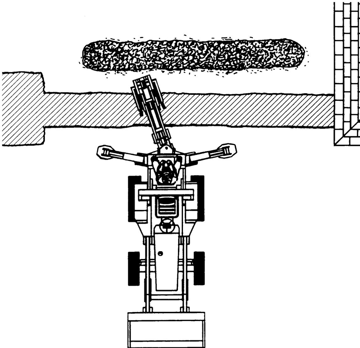
Position the unit forward so the two trenches can be connected. Pile the spoil on the opposite side of the trench.
