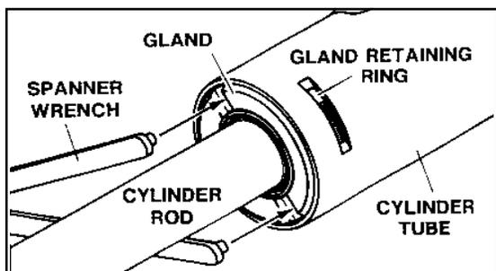
Pry up the end of the gland retaining ring with a pointed tool. Rotate the gland with
