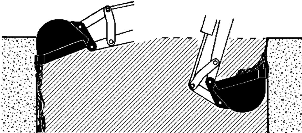
Once the sides are cleaned up, finish grading the bottom of the excavation. This is done by making the remaining cuts long and shallow, concentrating on making them level and smooth. Remove any remaining spoil. Check the excavation bottom for depth and levelness, making any adjusting cuts as needed.
