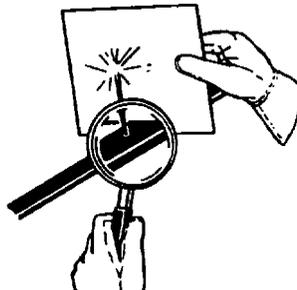
Physically check all pins, bushings, cotter pins, nuts, etc., for signs of wear or loose fit. Tighten as required, replacing where necessary. (Bolts and pins may vibrate loose during operation.) Clean equipment of all dirt, oil, and excess grease. This will assist you in making visual inspection and help avoid overlooking worn or damaged components.
