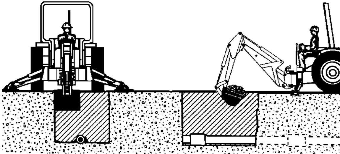
To check for pipeline leaks, start by digging a bellhole about six feet wide and ten feet long. Then, dig lengthwise along the pipeline to locate the leak. Once the leak is located, position the unit to dig at grade level on both sides of the pipeline. If a section of pipe is to be replaced, strip the soil from both ends of the bellhole. Enlarge the hole enough to allow the workmen adequate working space in the leak area.
