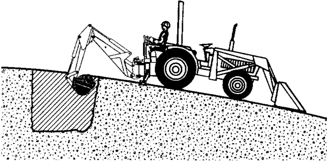
When digging on slopes always face the backhoe upgrade whenever possible. It may be necessary to cut a level surface in the hill for the backhoe to sit in when operating on slopes. This will allow the backhoe to sit level for digging the main excavation. Pile the spoil from the surface downhill. When digging the main excavation, pile the spoil uphill.
