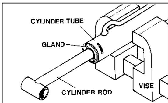
2. Rotate the gland with a spanner wrench (available from your dealer) until the gland retaining ring appears in the milled slot.
