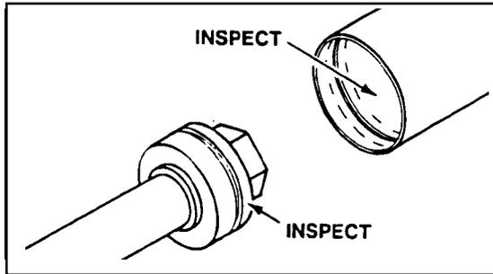
4 Remove the hex nut, piston, flat washer or spacer tube (if so equipped), and gland from the cylinder rod. If the cylinder rod is rusty, scratched, or bent, it must be replaced.
