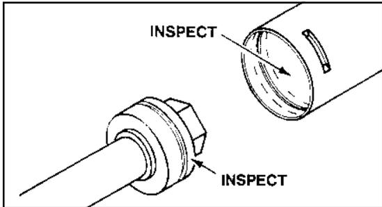
5 Remove the hex nut, piston, flat washer or spacer tube (if so equipped), and gland from the cylinder rod. If the cylinder rod is rusty, scratched, or bent, it must be replaced.
