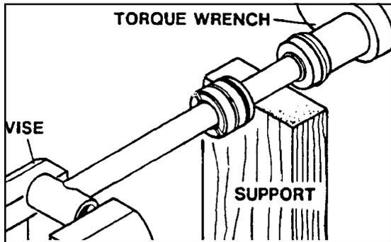
**IMPORTANT:** Do not contact the active surface of the cylinder rod with the vise. Damage to the rod could result.
