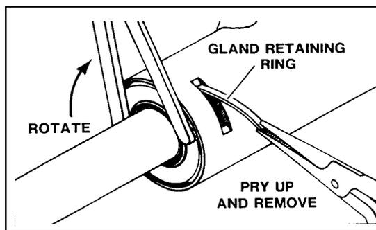
a spanner wrench while removing the retaining ring.
