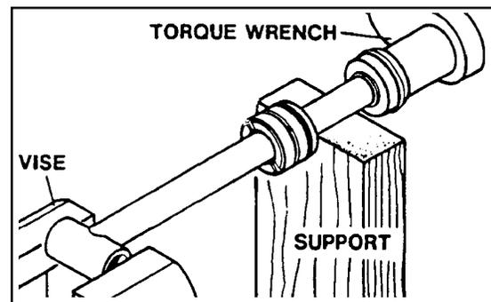
gland retainer ring should be hidden (not turned so it is exposed in the slot) to prevent it from popping out.
