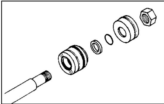
3 Secure the cylinder rod (mounting end) in a vise, with a support at its center. Torque the nut to the amount shown for the thread diameter of the cylinder rod (see chart).
