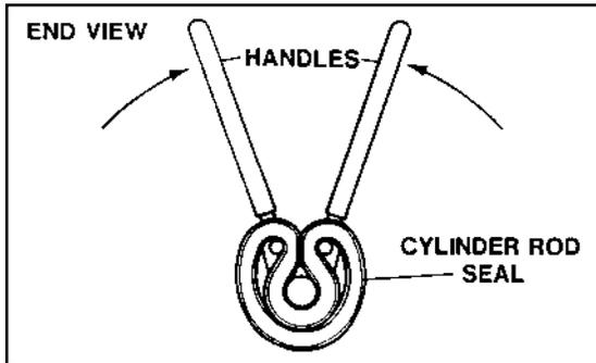
Now insert the seal into the gland from the inner end. Position the seal in its groove, and release and remove the tool. Press the seal into its seat the rest of the way by hand.
