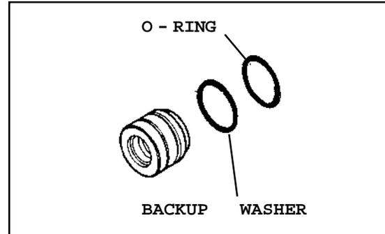
2 Slide the gland onto the cylinder rod being careful not to damage the rod wiper. Then install the spacer, or flat washer (if so equipped), small O-ring, piston, and hex nut onto the end of the cylinder rod.
