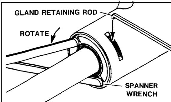
Rotate the gland until the gland retaining rod forms a ring between the gland and the cylinder tube.
