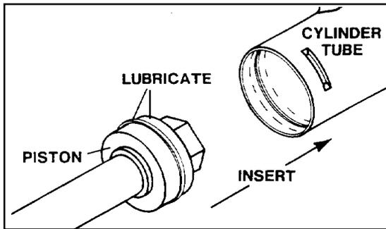
**IMPORTANT: Ensure that the piston ring fits squarely into the cylinder tube and piston groove, otherwise the ring may be damaged and a leak will occur.**
