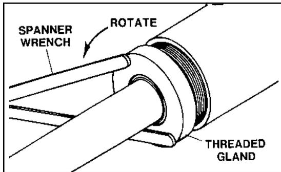
2 Pull the cylinder rod from the cylinder tube same as shown with the retaining ring type gland.
